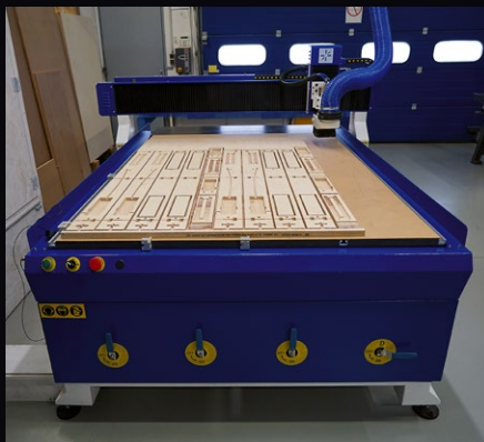
CNC milling machine for all MDF and plywood parts.
