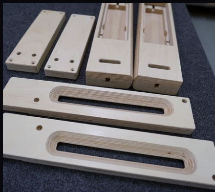
Plywood parts after machining and manual finishing.
